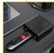
The built-in USB port allows easy connection to a data storage device.
